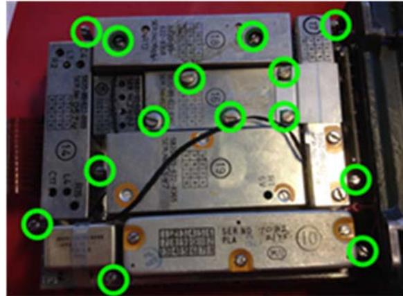
Note that the two bolts within module 18 should remain in place and the 5 screws in module 16 are screws not bolts and the little plate needs to be removed as well.. Note also that the bolt by assembly 17 is longer than the others (below left). Carefully unplug the RF connector linking the two halves as shown below centre, then the top half should fold away from the frame as shown below right.
