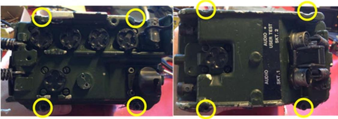
Remove the remote panel by unplugging it from the main body as shown in the picture on the right, then removing the case as shown below.
